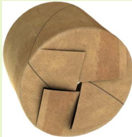
Paper tube 4 cuts, then fold over
